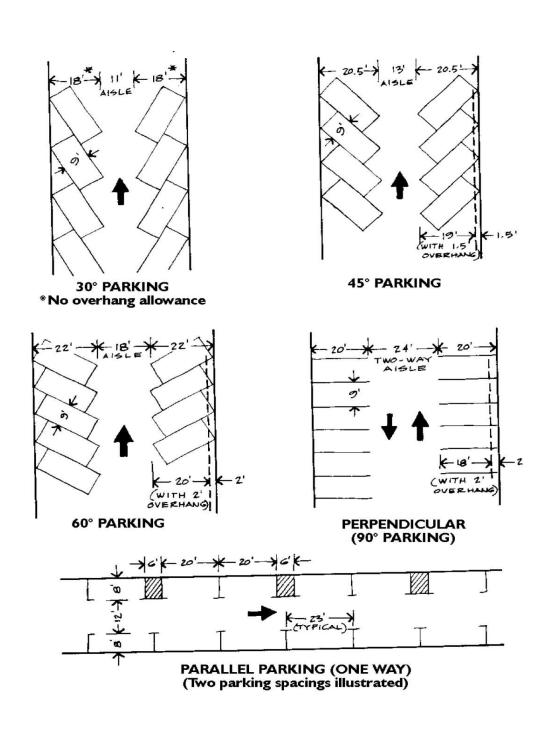
**NOTE:** In parking garages only, perpendicular 90 degree stalls/spaces shall require a width of nine (9') feet and a length of eighteen (18') feet.
